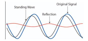
Reflected power from a mismatch comes back down the feed line on the outer jacket of the coax. This reflected RF power can "bite" the operator and may result in reports of garbled, distorted, or unintelligible voice transmissions
