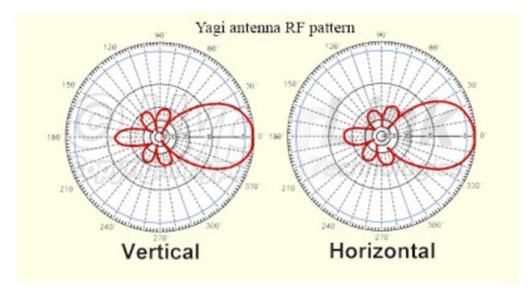
To focus the beam in the vertical: add elements to the beam To focus the beam in the horizontal: stack another yagi
