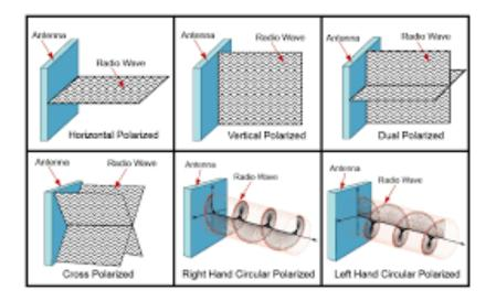
When working long distances or with weak signals, a horizontal polarization generally works better because most interference (nature made and man made) has vertical polarization
