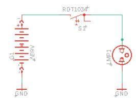
1. If the voltage in this circuit is 13.8 volts DC and the current is 10 amperes, how much power is being consumed?
